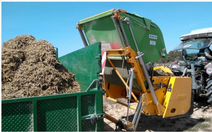
The Cobra Collina (by Peruzzo) unloads vineyards pruning chips to a trailer
