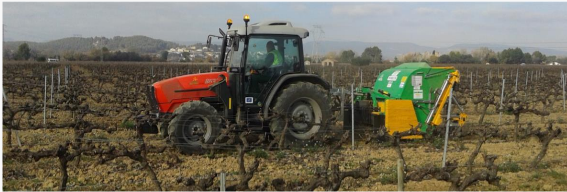
Harvesting + pre-treatment process using the Cobra Collina
